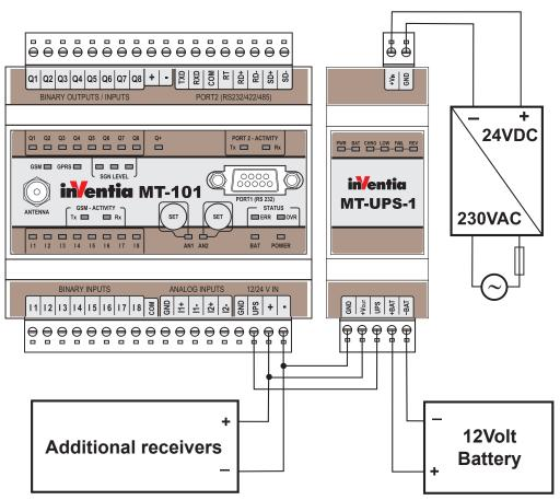
An example of connection of MT-UPS-1 to MT-101 telemetry module
