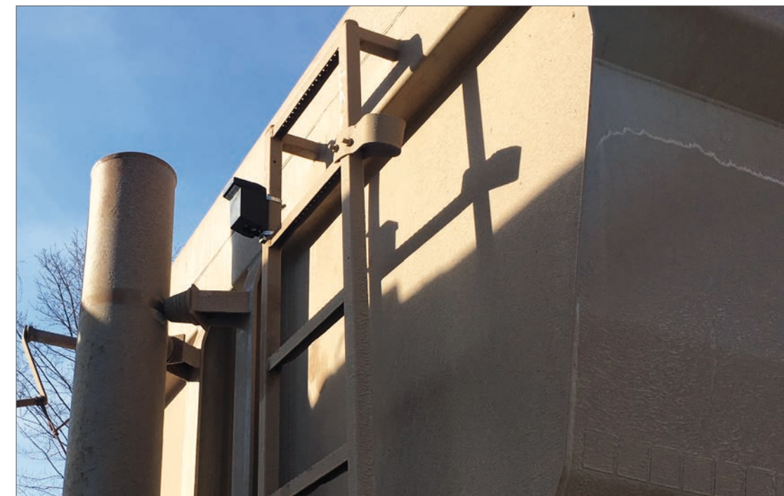
Trailing and unloading sensor mounted on the trailer
