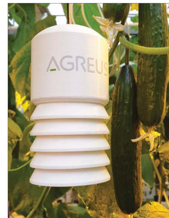
Fig. 3 Air temperature and humidity sensor AM-200
