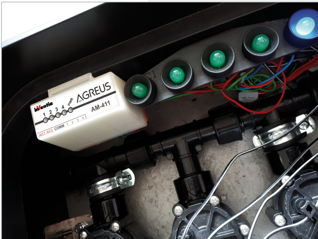
The photo above shows the base station responsible for communication between system elements located in the field and computing cloud. The valve control module and the control panel of the valve station are presented below.
