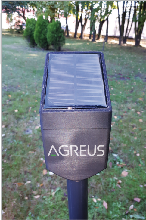
The pictures show the components of the AGREUS system. Above the soil probe is shown, i.e. humidity, temperature and salinity sensor. Field temperature and humidity sensor is shown below.
