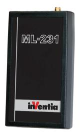
ML-231 is a specialized telemetry module dedicated to monitor status and location of vehicles. Module's design is based on latest GPS/GSM technologies securing precision of localization and GSM signal propagation. The design complies with automotive industry design standards.
